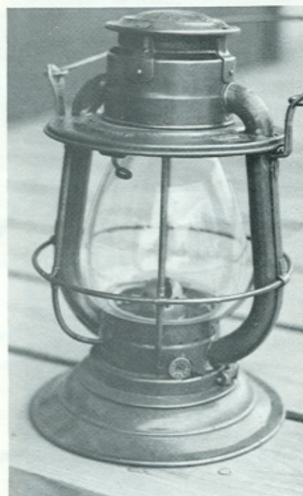
Dietz Vesta Lo-top Bell Bottom 4 1/4" globe. Overall height 10", font twist off bell 6 1/2" dia. 1-5/8" high, across top of burner at inside of tubes 4 1/2", across at horizontal wire 4-13/16", across at top of tubes 3-15/16".
