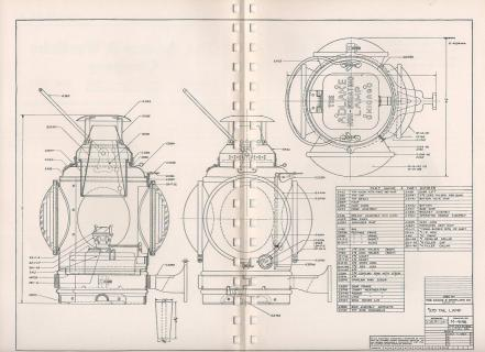
ADLAKE SQUARE TOP NON-SWEATING BALANCED DRAFT VENTILATION has proved superior to all other types of signal lamp ventilation in over twenty years of satisfactory service. It is made of heavy drawn steel, dipped in terne metal and the parts are easily removable for cleaning.
