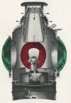
ADLAKE WIND-PROOF DOOR increases the efficiency of Adlake Square Top Ventilation. A heavy pressed steel door frame adds strength and rigidity to the door assembly. Weatherstrips are added around the door and wick raiser. See Bulletin B-31 for further details.
